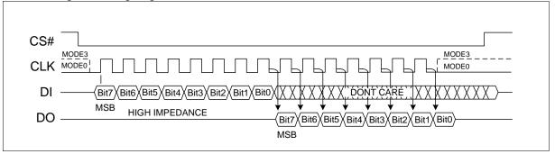
Figure 2 The difference between Mode 0 and Mode 3
